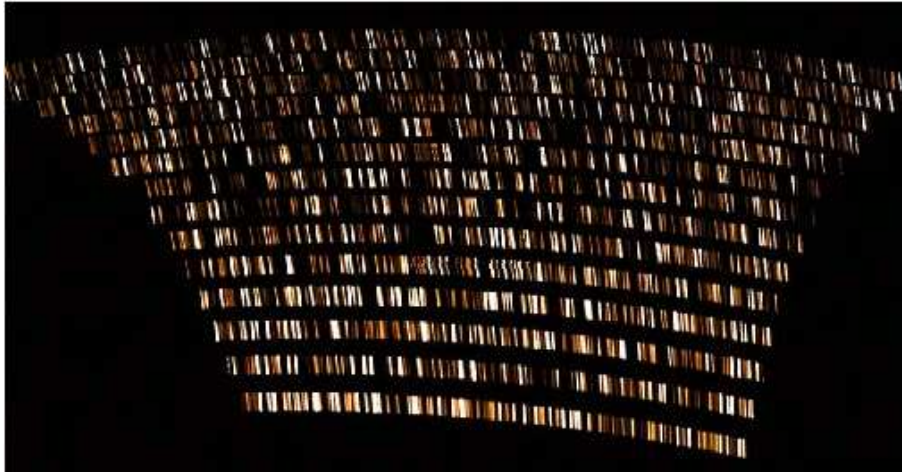
Figure 10.8: Simulated spectrum of a ThAr lamp through the VIS spectrograph.
